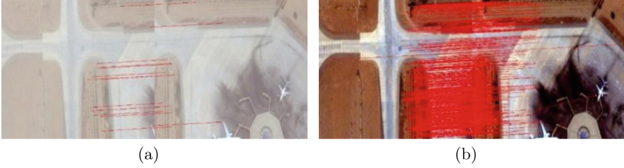
Fig. 3. A group of example images in the keypoint matching task (with RANSAC). (a) Before the haze removal, 19 keypoint pairs are matched. (b) After the haze removal, 744 keypoint pairs are matched.
