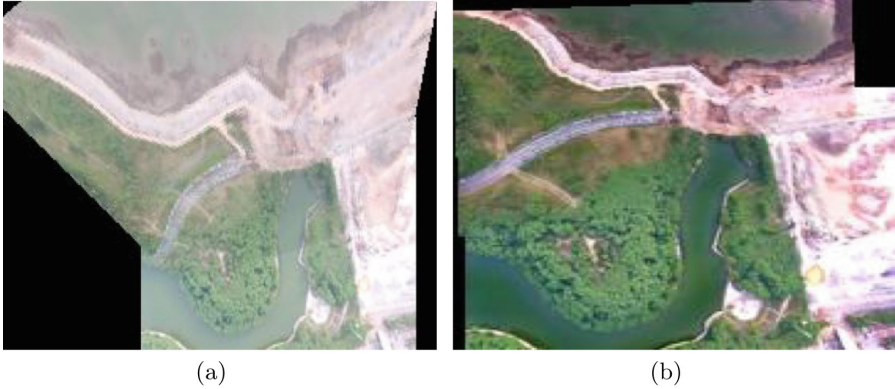
Fig. 7. A group of example images in the image stitching task. (a) is the result before haze removal, and (b) is the result after haze removal.
